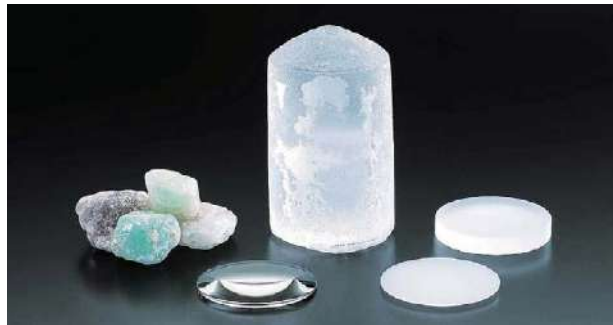
Natural fluorite (left) and artificial fluorite crystal (centre)
